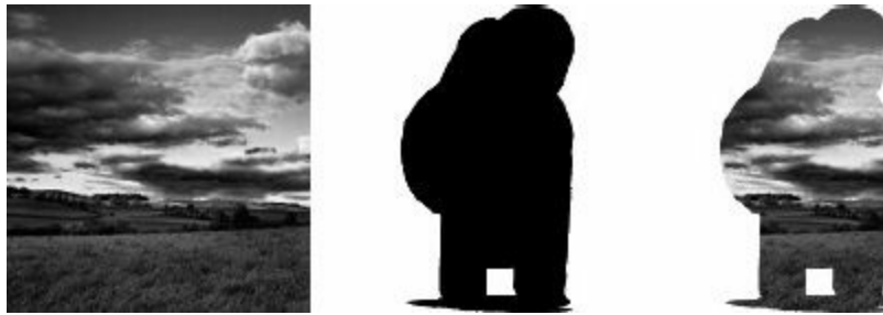
Figure 8-10. From left to right, a background, an image mask, and the mask applied to the background
