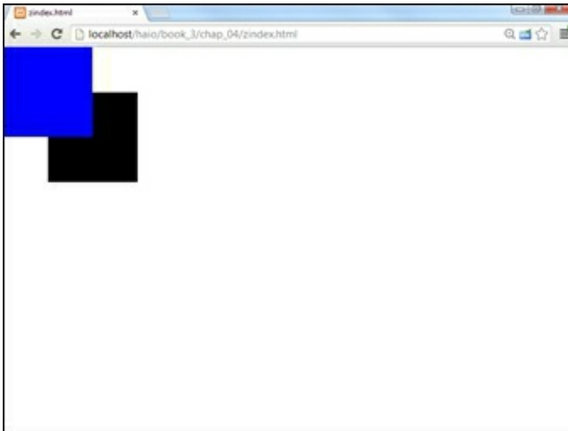
Figure 4-3: The z-index allows you to change which elements appear closer to the user.
