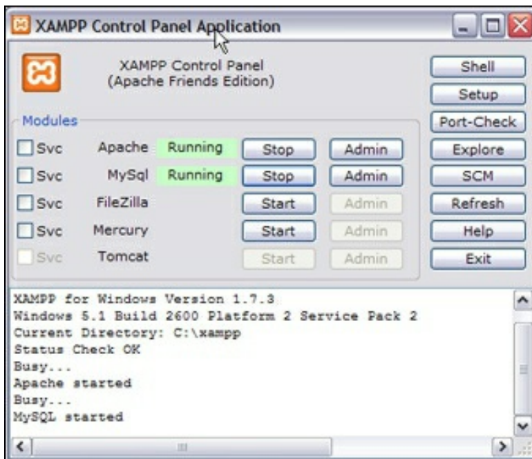
Figure 1-2: I've turned on Apache and MySQL in the XAMPP control panel using the buttons.
